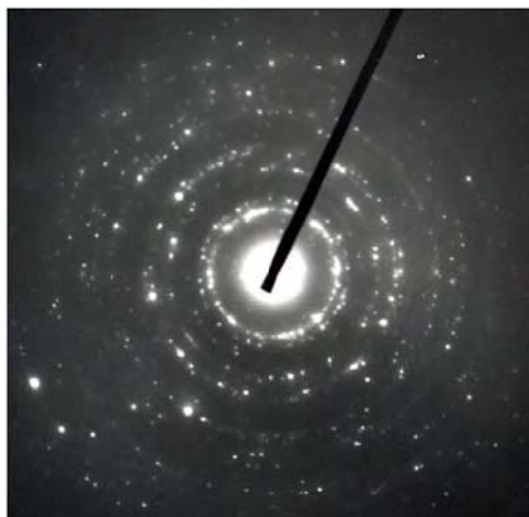
Figure 2.20: Electron diffraction pattern of a typical polycrystalline nanowire.
